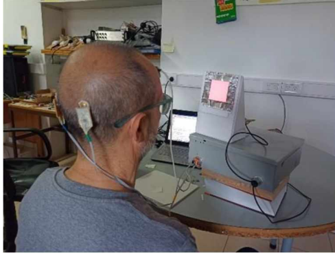
Fig. 5. Experimental setup. The measurement electrodes, DRL on the forehead, and stimulator are observed.
