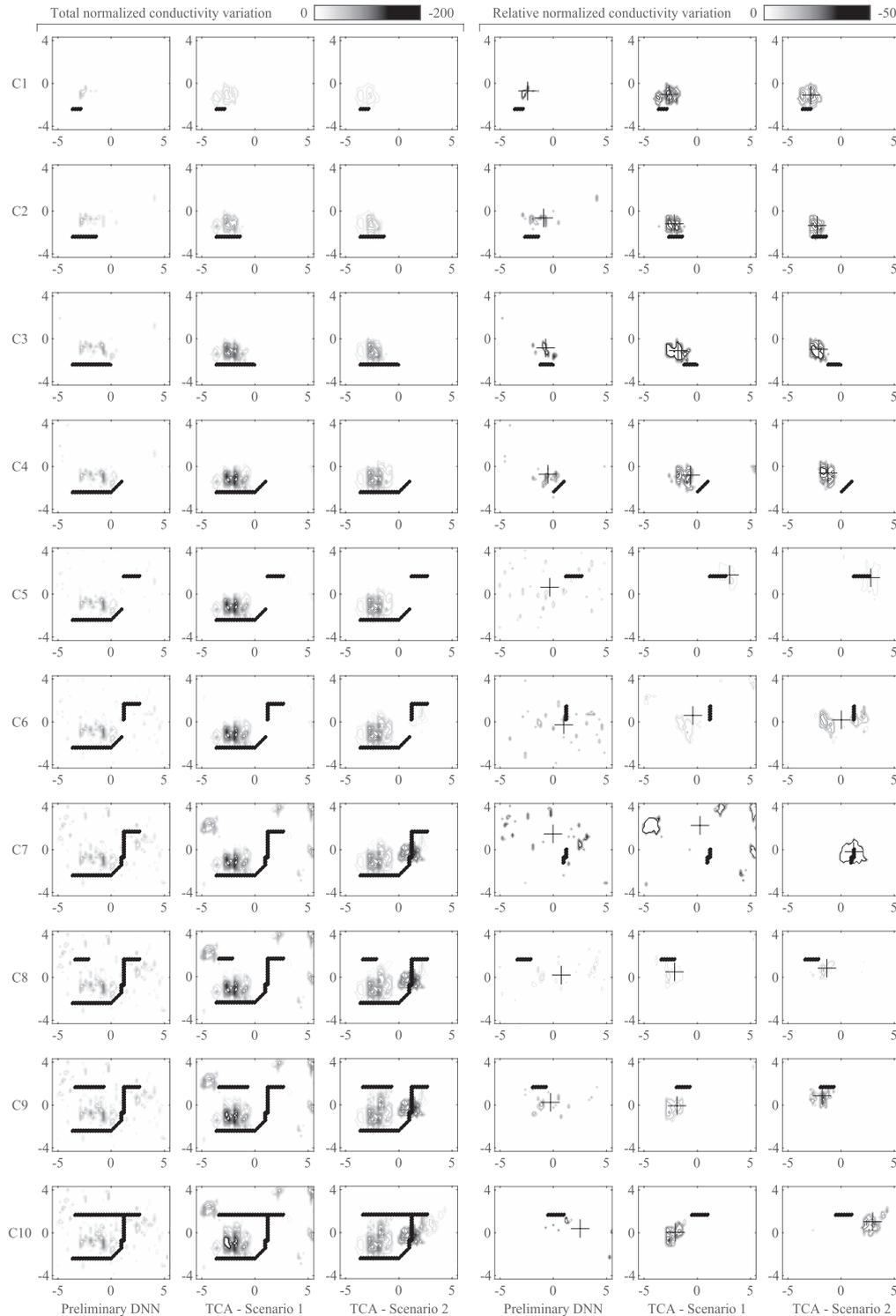
**FIGURE 11** Experimental results for specimen 2. Left: total normalized conductivity variation; right: relative normalized conductivity variations. The gray contour depicts the identified conductivity, + symbols represent their centroids, and thick black lines are the reference cracks.
