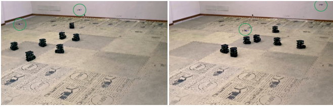
Figure 9. Snapshots from the second experiment. Left: robots have reached the pickup positions and perform the loading operation (simulated). Right: robots have reached the delivery positions and have terminated the mission.
