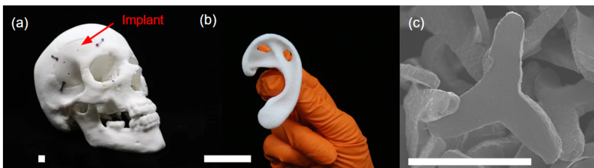
Figure 1.1 (a) StarPore® cranial implant placed within a human skull model, scale bar = 10 mm, (b) StarPore® human ear implant, scale bar 25 mm, (c) StarPore® trilobal HDPE particles used within the implant, scale bar = 1 mm.
