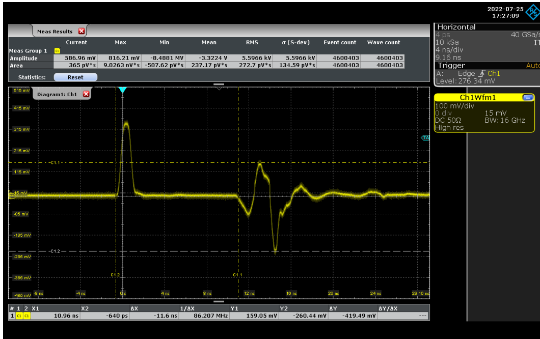
Figure D.2: Oscilloscope trace for the generated spike of the 4.5 \mu\text{m} RTD, when disturbed in its reverse valley voltage. The bias voltage was of -1.52 \text{ V} and the pulse amplitude was of 350 \text{ mV} and 1 \text{ ns} width.
