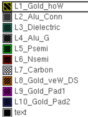
Figure B.1.: PDK available layout layers and coloring.
