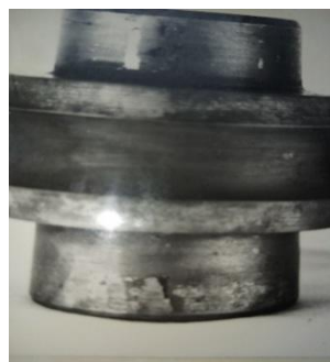
Fig. 5. Chipping of rollers
