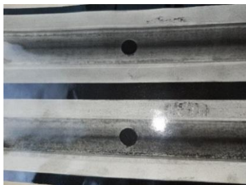
Fig. 3. The nature of the distribution of wear along the length of the working track of the bar
