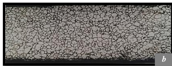
Fig. 1. Microstructure of finished (5.8×0.3 mm) tubes: regular technology (a); intensive technology (b) ×100
