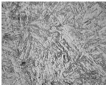
Fig. 2. Microstructure of the blade metal upon the bulk heat treatment, ×100
