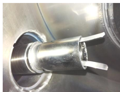
Fig. 9. Anti-spatter UHF input after 20 hours of operation in Ar GD
