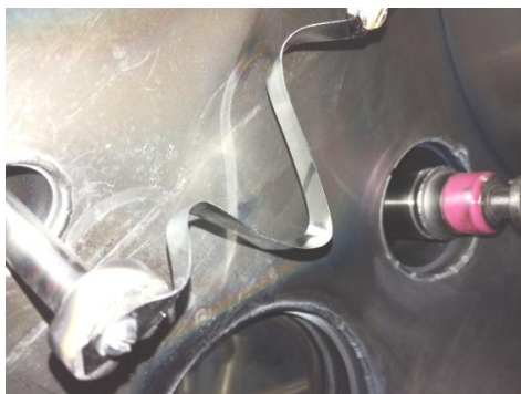
Fig. 4. Thermal desorption SS probe in situ in the DSM-1 vacuum chamber
