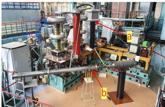
Fig. 7. Photo of the bench assembly: a – T-10 HIBP high-voltage power supply; b – test bench
