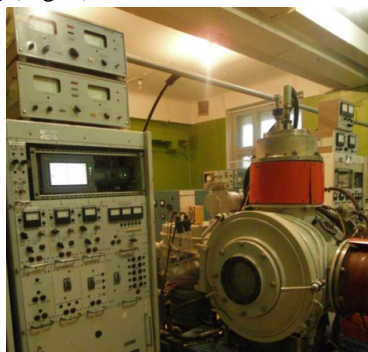
Fig. 1. Appearance of the "Bulat-6" installation (control rack with controller and vacuum chamber)
