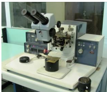
Fig. 9. The microwelding installation US.IMM-1 (equipment used in the former USSR)
