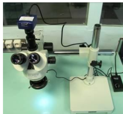
Fig. 10. KONUS CRYSTAL PRO stereo microscope with digital video camera Levenhuk M800 Plus
