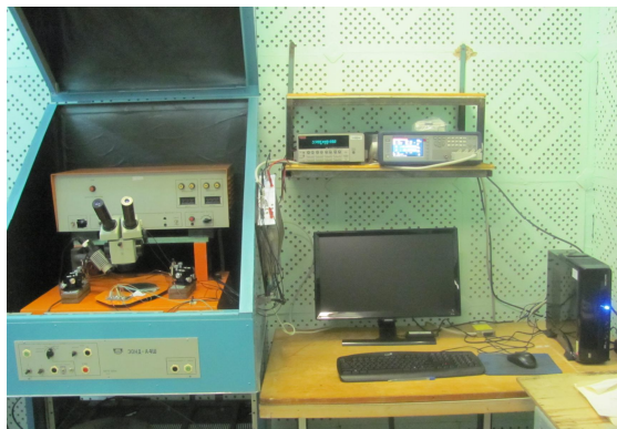
Fig. 2. General view of the automated test station with the automated movement of microprobes and the automated storage and processing of measurement data of detector electrophysical characteristics
