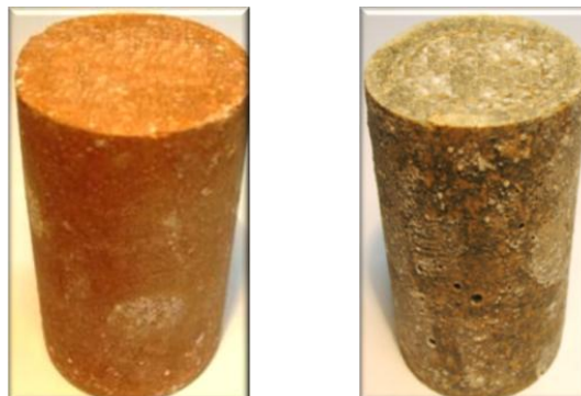
Fig. 9. Solidified simulators of the KW and KE Basin sludge waste
