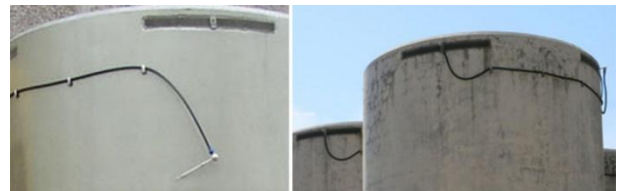
Fig. 2. Resistance thermometer and the place of its location in the system of thermal monitoring
