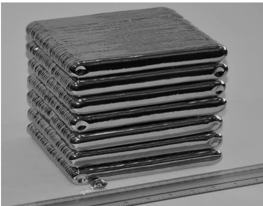
Fig. 3. Appearance of flat tungsten single crystals 170x160x20 mm
