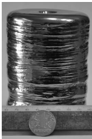
Fig. 7. The appearance of a tungsten crystal with a diameter of 85 mm
