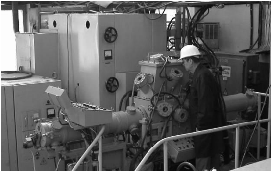
Fig. 2. The equipment for growing single crystals of refractory metals in the form of plates
