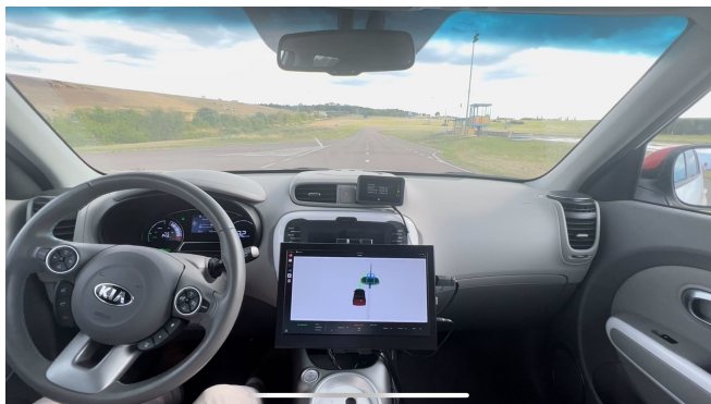
Fig. 1: Validation of the MPPI-based motion planner on a closed track using a modified KIA Soul EV equipped for autonomous driving. The figure depicts the object avoidance scenario whereby a virtual object was placed on the path.
