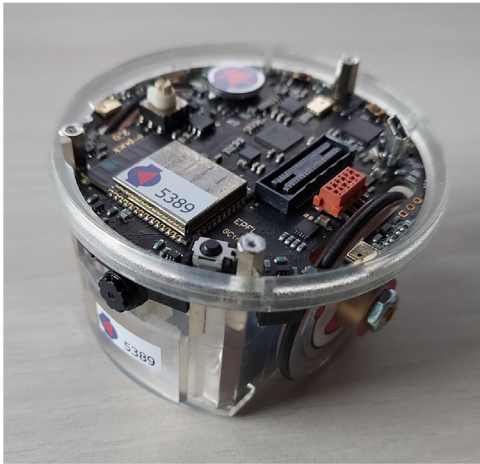
Fig. 1. The E-Puck2 robot (E-Puck version 2).
