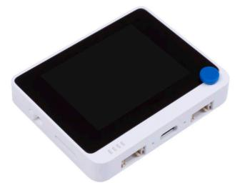
**Figure 5.** Wio terminal as the second RTU.
