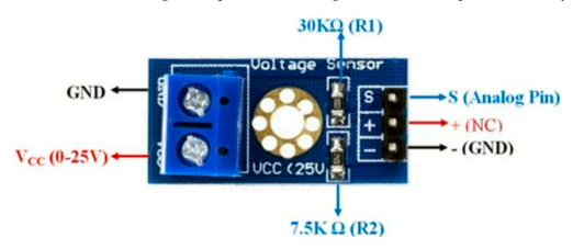
Figure 3. F031-06 voltage sensor module.
