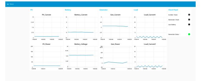
Figure 13. Node-Red dashboard for visualization.
