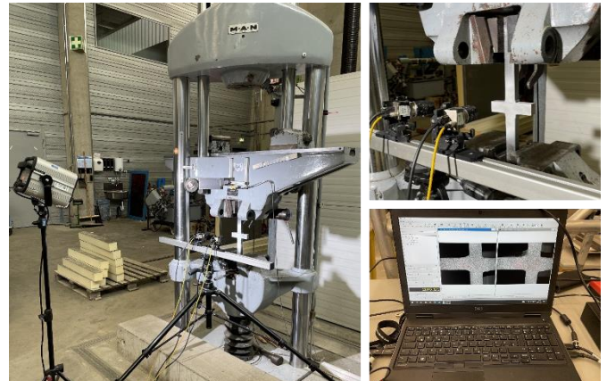
Figure 9 Tensile tests on cross joint specimens - experimental setup
