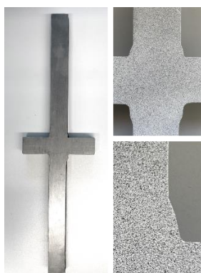
Figure 8 Prepared test specimens with a stochastic pattern
