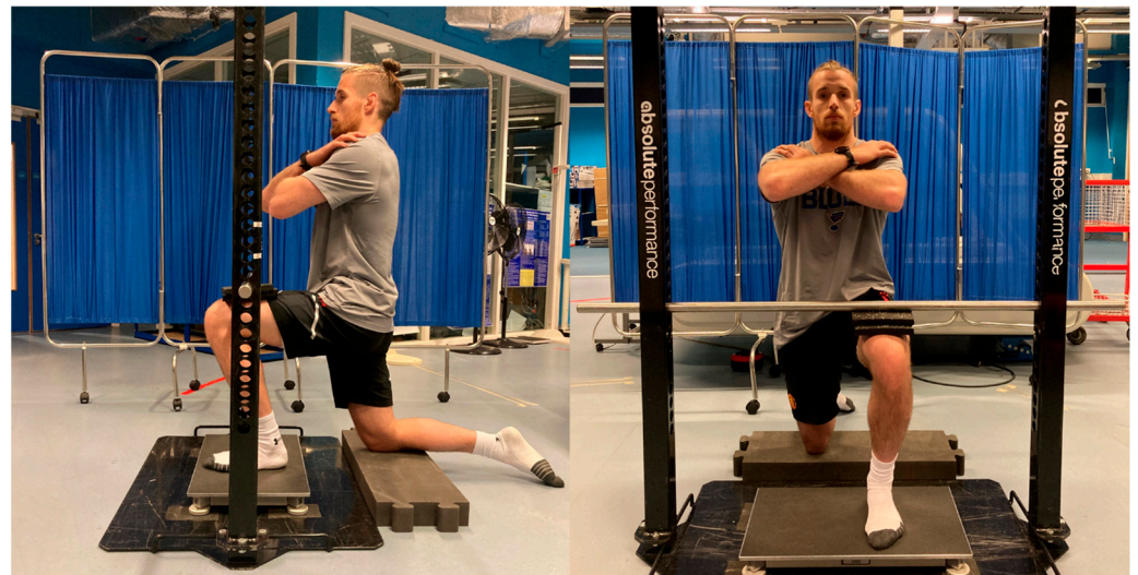
Figure 1. The sagittal (left image) and frontal (right image) view of the kneeling isometric plantar flexor test to illustrate the equipment and participant positioning.
