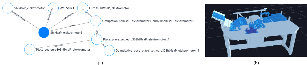
Fig. 3: Graphical representations of ontological knowledge. (a) shows entities (circles) and their properties (lines) that are modeled in the ontology. The example shows a physical object marked as blue dot ( Artifact ) of a specific type ( \rightarrow idealizedByDesign \rightarrow Design ) and how it is geometrically ( \rightarrow spatialParent \rightarrow Storage ) and semantically ( \rightarrow causes \rightarrow Occupation \rightarrow ofPlace \rightarrow Place ) referenced in the ontology. (b) Visualization of the variable workstation.
