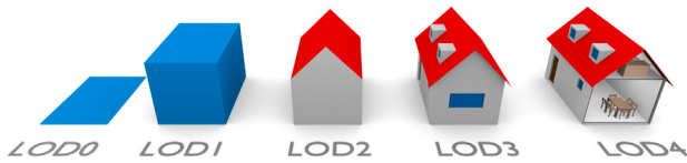
Fig. 4. The five different LODs for building models in CityGML 2.0 (Biljecki et al., 2016). Licensed under CC BY-NC-ND 4.0.
