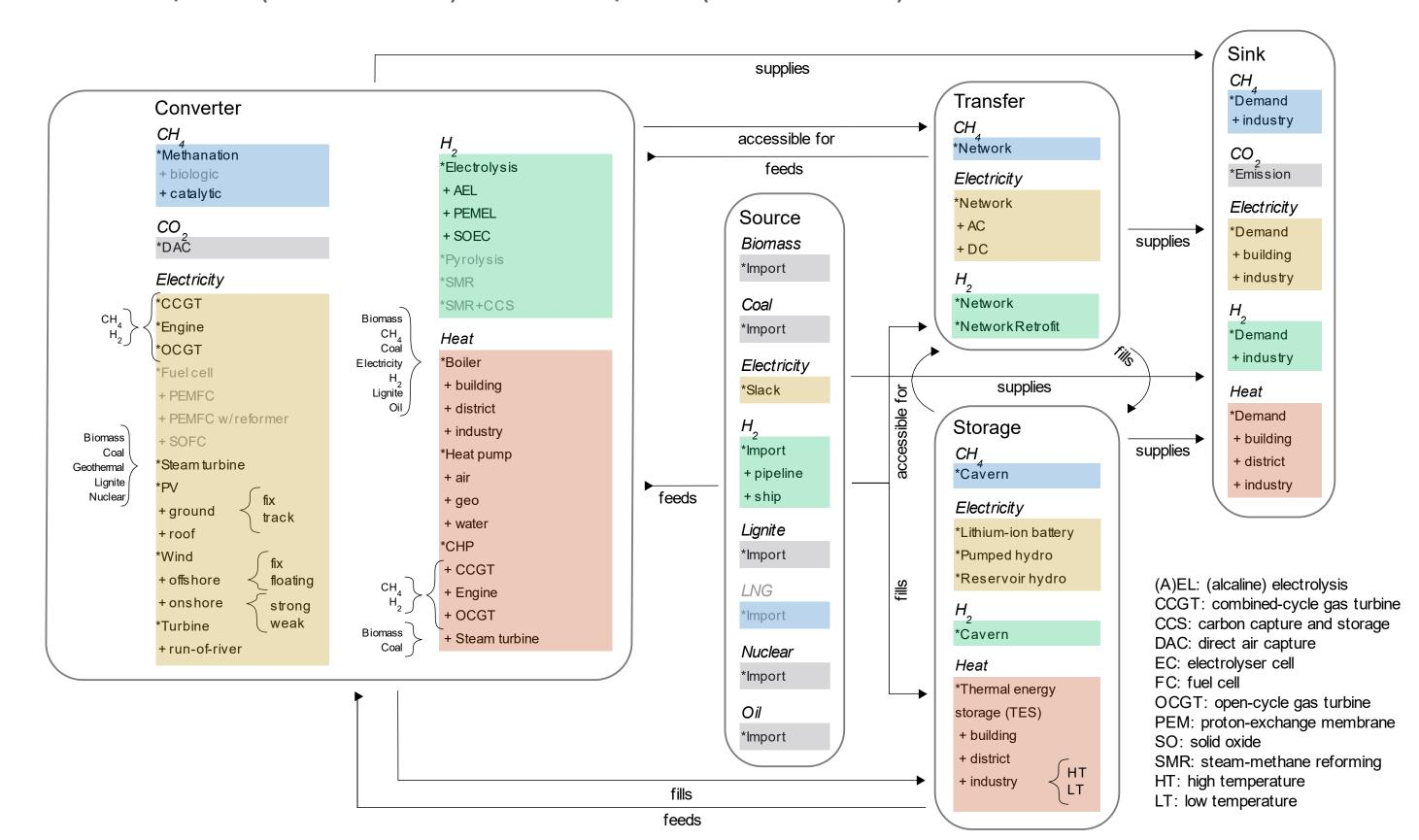
Figure 2 - Technological scope (own visualisation): more than 90 technologies in the model.
