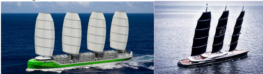
Figure 2: Shown above are two examples of soft sails, on the left is the Ecoliner concept rendering from Dykstra while on the right is the Black Pearl sailing vessel which was delivered by Oceanco in 2016. Both vessels feature a Dynarig setup.
