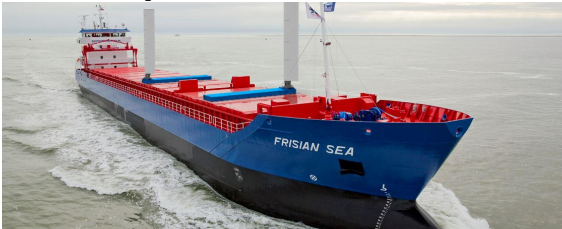
Figure 5: the FRISIAN SEA utilizes two Flatrack suction wings
