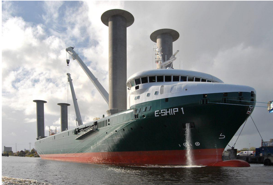
Figure 3: Shown above is the E-SHIP 1 which is a general cargo ship utilizing Flettner rotors. This particular ship is used for transporting wind turbine components.
