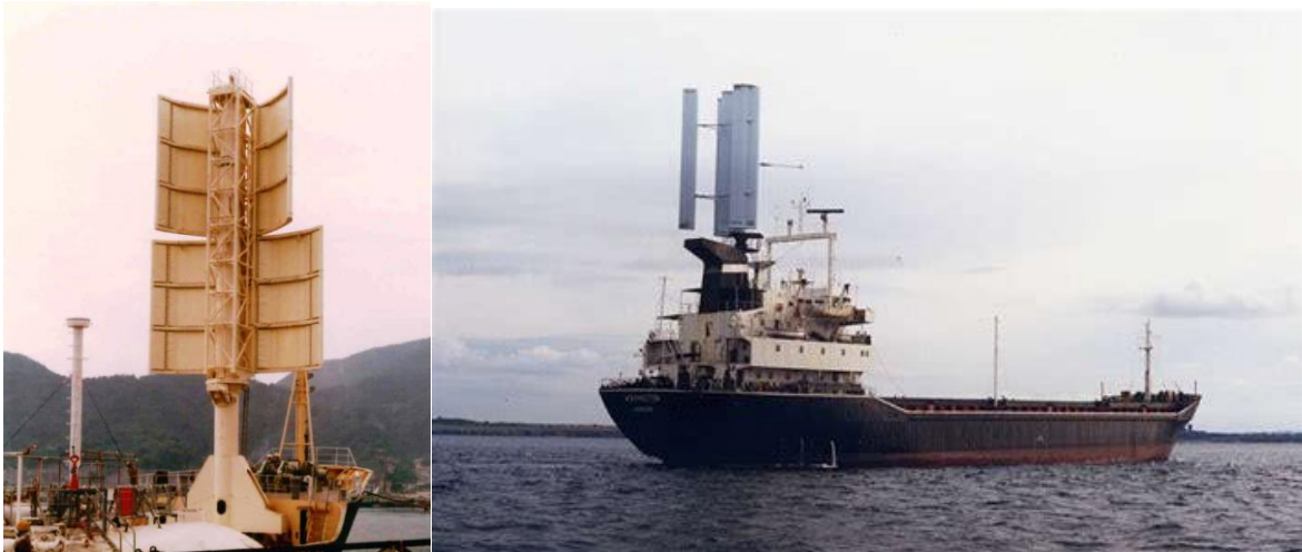
Figure 1: Shown above are some of the first commercial examples of rigid sails in use. On the left is the JAMDA sails and on the right the MV Ashington which is outfitted with the Walker WingSail.
