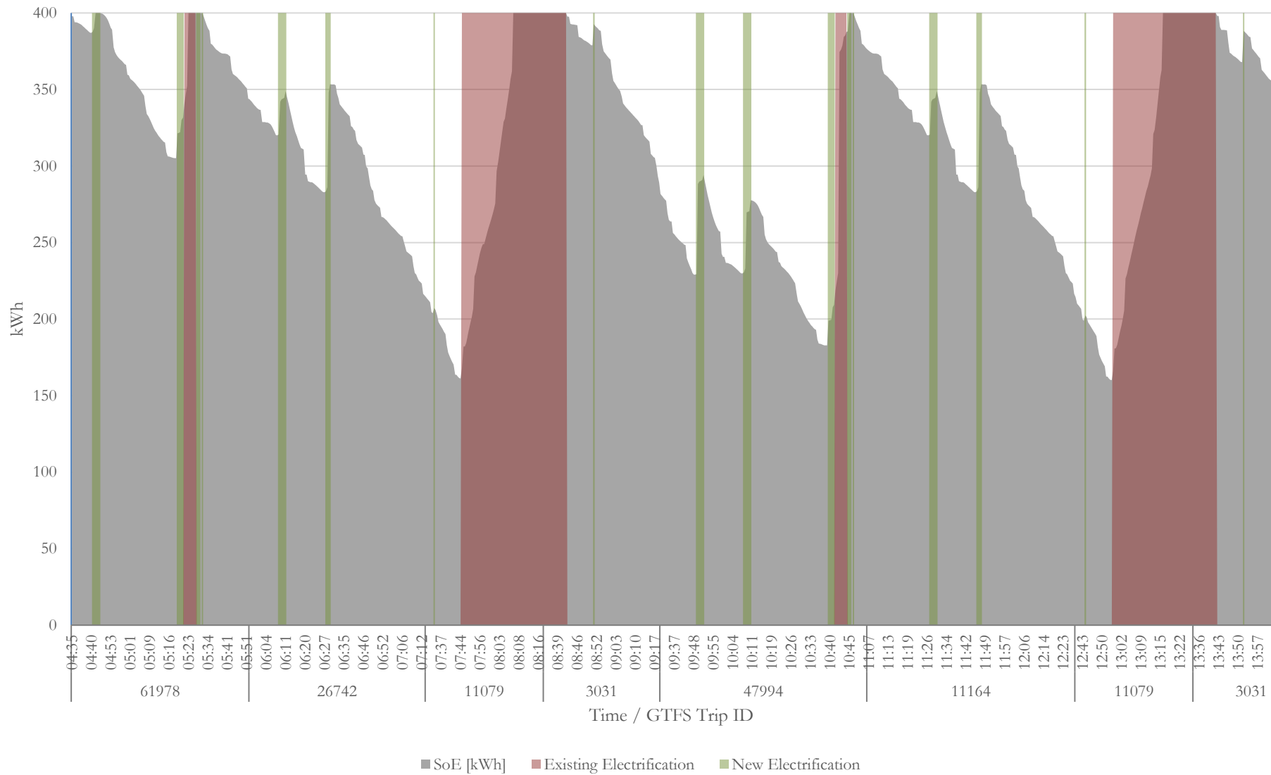
Figure 101: State of energy and the presence of electrification for vehicle 156632710 through its circulation given the distribution of existing and new electrification within the results of model run “standard substation 2”.
