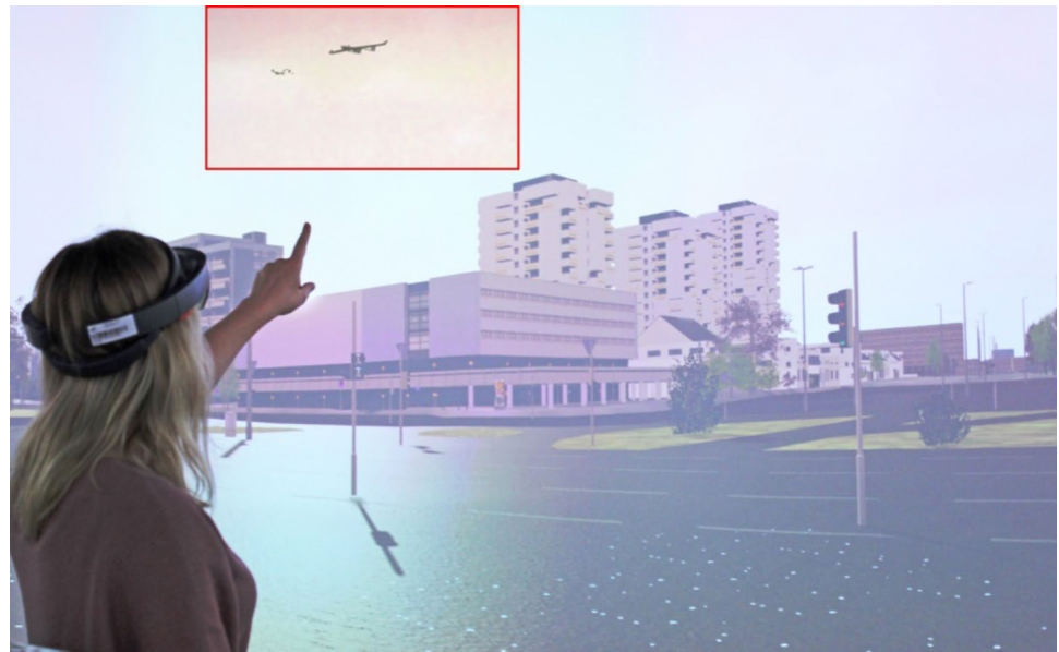
Fig. 4 Participant watches the scenario through the HoloLens in the VR Lab. The red square highlights the visualized drones seen through the AR-headset
