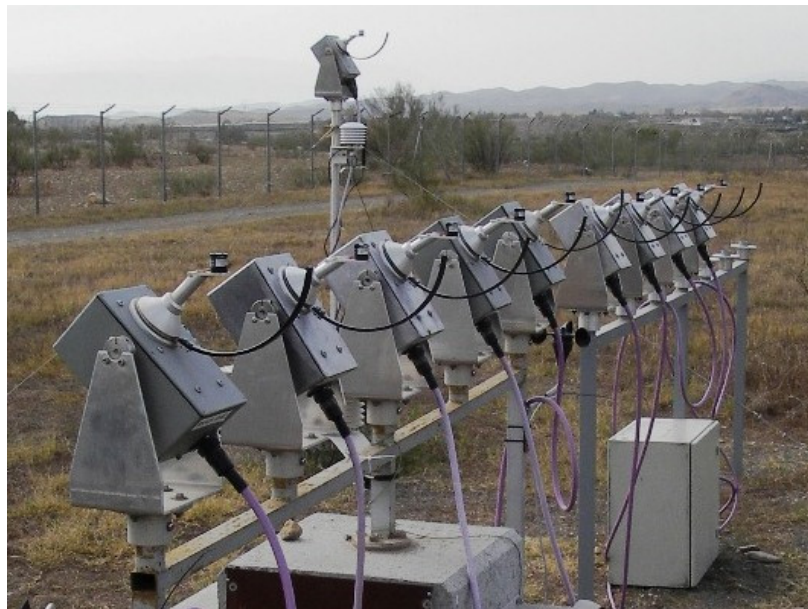
Figure 18: RSI calibration mount of DLR at CIEMAT's Plataforma Solar de Almería.
