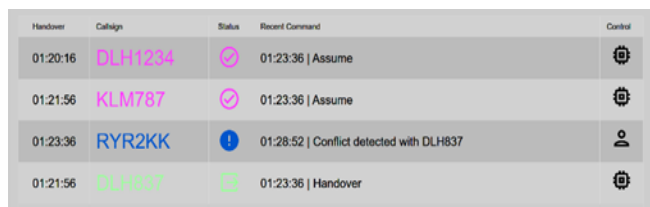
Figure 17 The flight strips in HI-DIRC give an overview of the current status of each flight, the most recent command or status update received by the flight, as well as the current control mode (human or digital ATCO)
