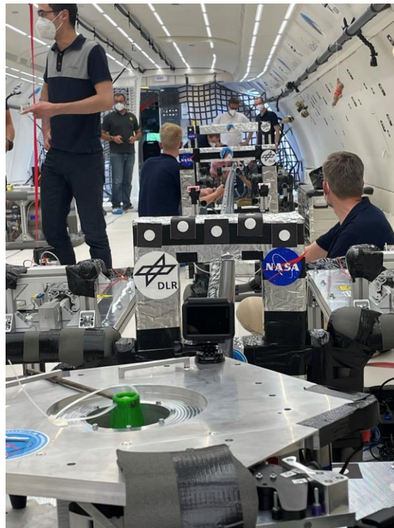
Fig. 5. Preflight testing of all test procedures inside the aircraft for in-flight operations. Image shows the deployer mechanism with the deployed boom passing through the center of the three rectangular safety gates.
