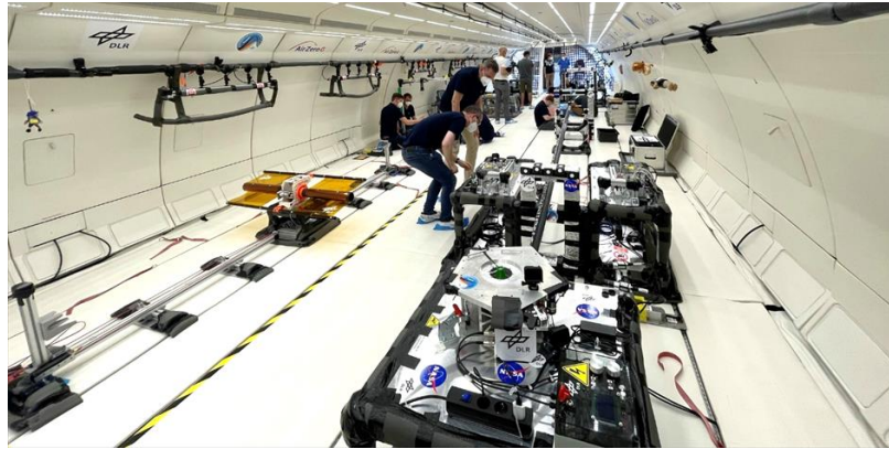
Fig. 10. Full test setup installed in the cabin after camera calibration.
