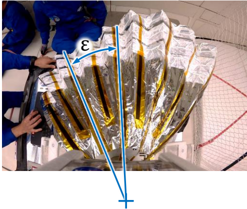
Figure 10: Flatness determined by image measurements of deployed wings.
