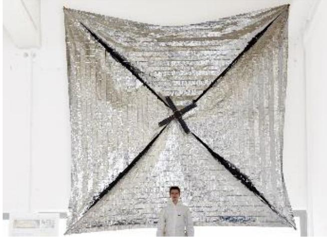
**Fig. 4 Functional model of DeorbitSail drag sail (Source: DLR).**
