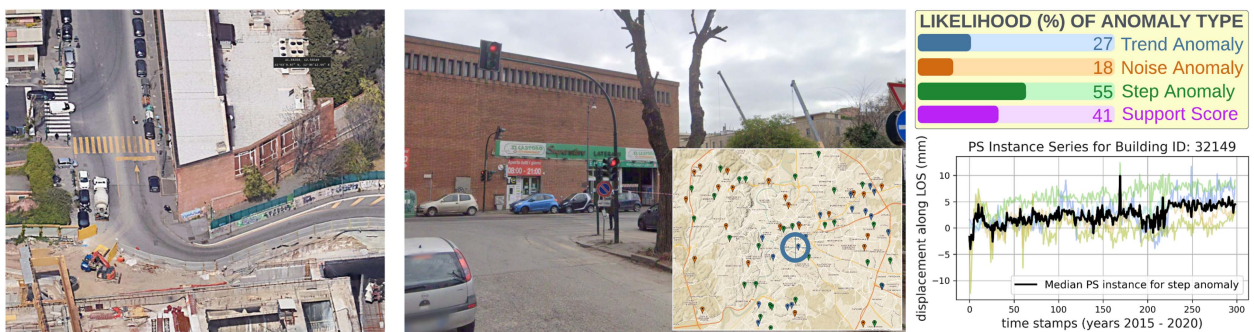
Fig. 17. Building with the detected anomaly of step . Empirical evaluation based on aerial views shows that the building is next to a subway construction site which might be a reason for the observed displacement.
