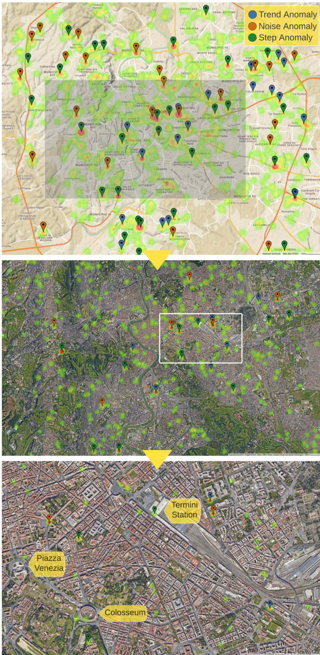
Fig. 14. Detected anomalies when the upper whisker threshold: 98%. Each location pin shows a displaced building with at least five anomalous PS instances. The heatmap shows the anomalous PS density per area.
