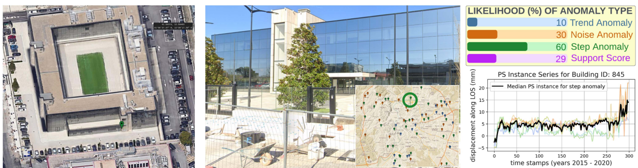
Fig. 18. Business center with the detected anomaly of step . Based on the aerial and street views, the center is newly built and there are ongoing landscape construction activities surrounding it, which could potentially explain the detected “displacement” in the area.
