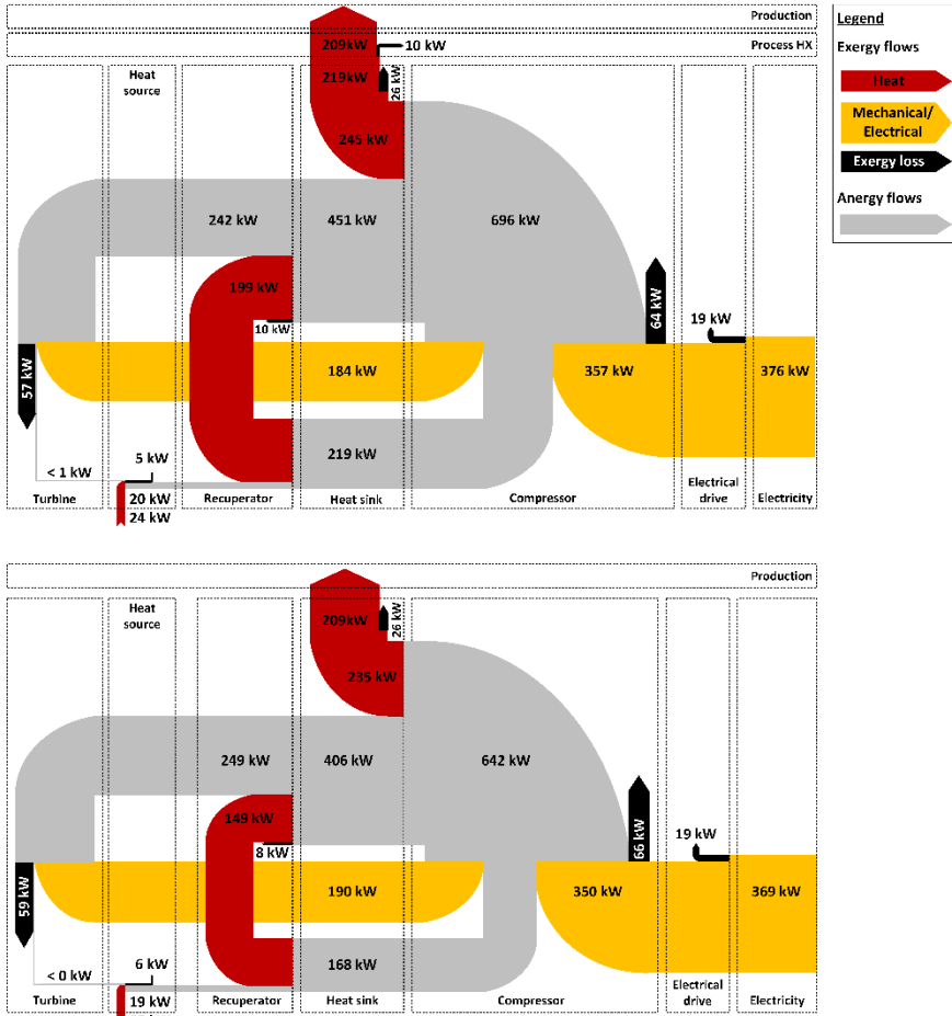
Fig. 2: Exergy analysis of the thermal oil integration (above) and direct integration (below)
