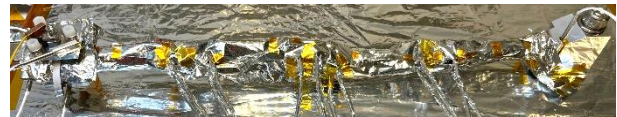
Figure 4: Experimental setup of single-lap joint on cold plate without (top) and with (bottom) SLI wrapping. A separate SLI (not shown) is enclosing the heater flange.
