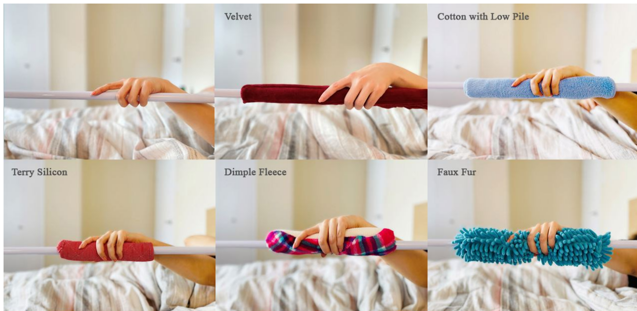
Figure 11: Photography documentation of haptic experiment with the designed fabric covers for the handrail of a patient bed
