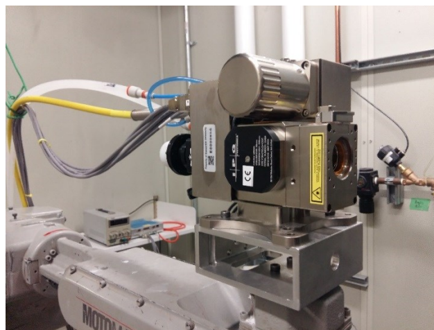
Figure 3-9 Robot-mounted 4 kW Laser used to remelt the top layers of the coating.
