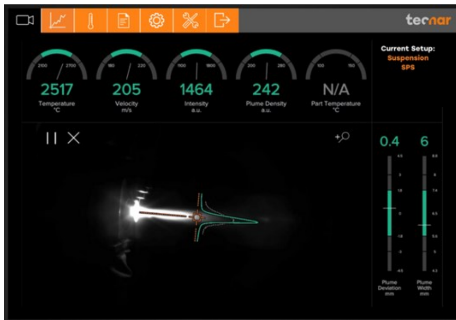
Figure 3-10 Examples of the outcome of an online monitoring of a plasma spraying process with Accuraspray [130].
