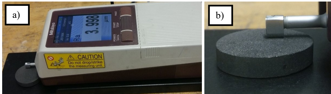
Figure 3-2 Roughness meter (a) and zoom on the measuring tip on a graphite substrate (b).
