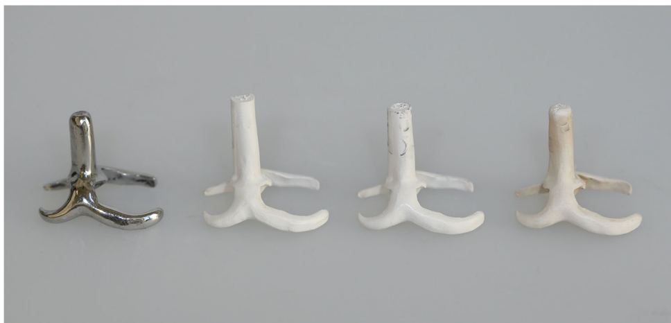
Fig. 2 RDP clasp specimens made of CoCrMo, PEEKmilled1, PEEKmilled2 and PEEKpressed
