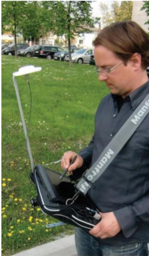
Figure 8.2 Tablet computer with GPS for outdoor AR(left) Georegistered view of virtual excavation revealing gas pipeline. [1]
