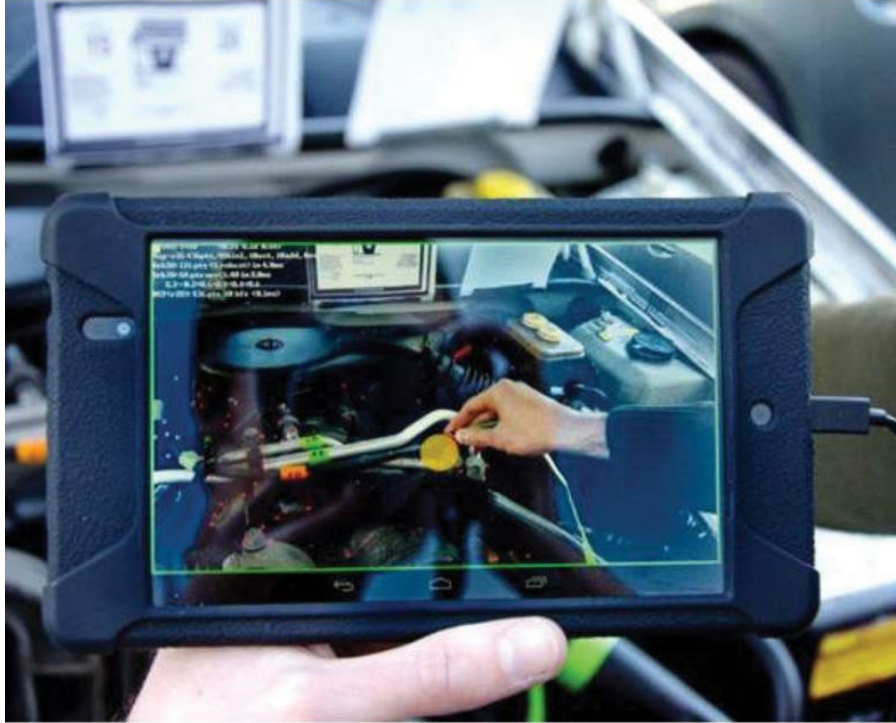
Figure 8.6 Using augmented reality telepresence on a tablet, a distant expert assists in an automobile maintenance scenario. [1]
