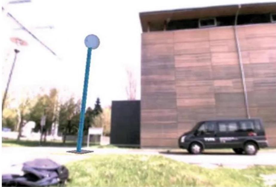
Figure 8.3 A spherical AR overlay can be used to visualize the drone's position even when it is far away and scarcely visible. [1]
