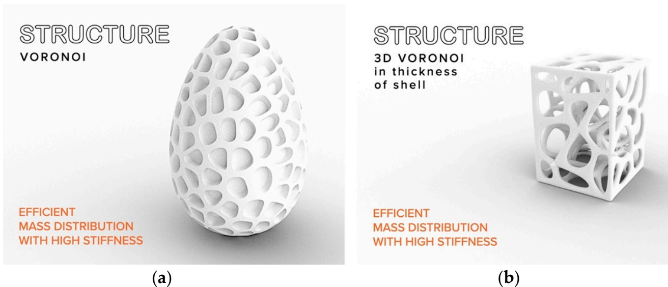
Figure 4. Generated model of the Voronoi structure: (a) implemented single-layer Voronoi structure on an egg-shaped surface, (b) cut-out of the 3D Voronoi structure that can be used for the entire outer wall thickness envelope.
