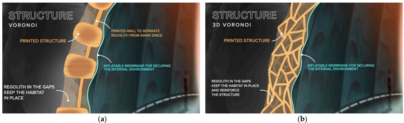
Figure 5. Schematic representation of the use of a Voronoi structure in cross-section view: (a) single-layer Voronoi structure with a partition wall, (b) 3D Voronoi structure with regolith infill.
