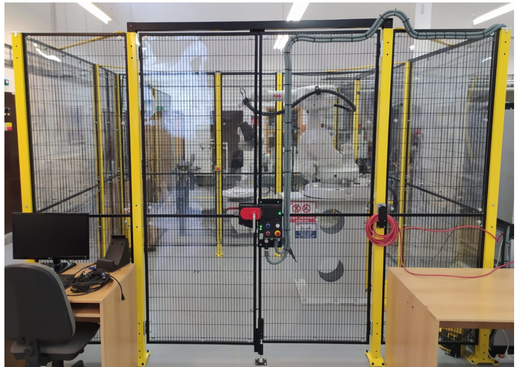
Figure 1. The picture shows a robot cell with an ABB IRB1600 robot.
