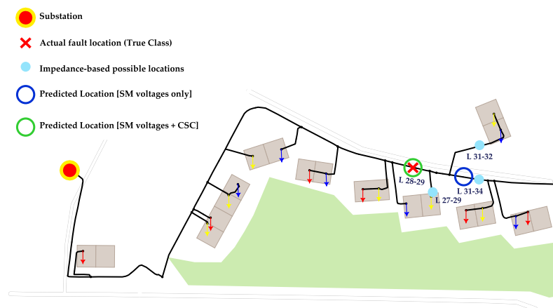
Figure 8. Comparison between fault location estimation through an impedance-based method, ML-based classification using SM voltages only, and ML-based classification when using SM and CSC.
