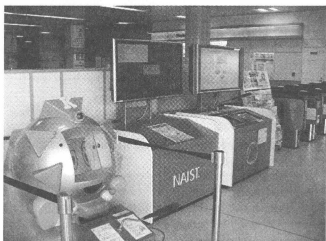
Fig. 2. Real-Environment Speech Train Information Guidance System "Kita-chan(back), Kitarobo(front)" : System installed at the local railway station since March 2006.
