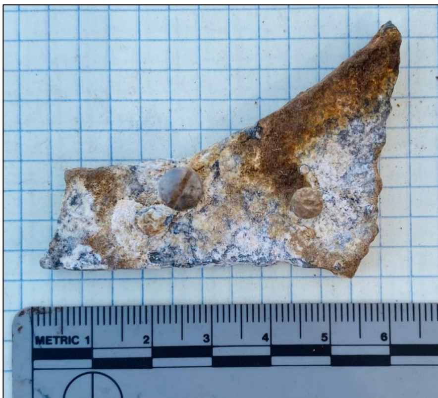
Figure 5.4. Fragment of corroded aluminum from the B-24's metal shell. The burning and subsequent corrosion of the aluminum has created the bluish-white appearance.
