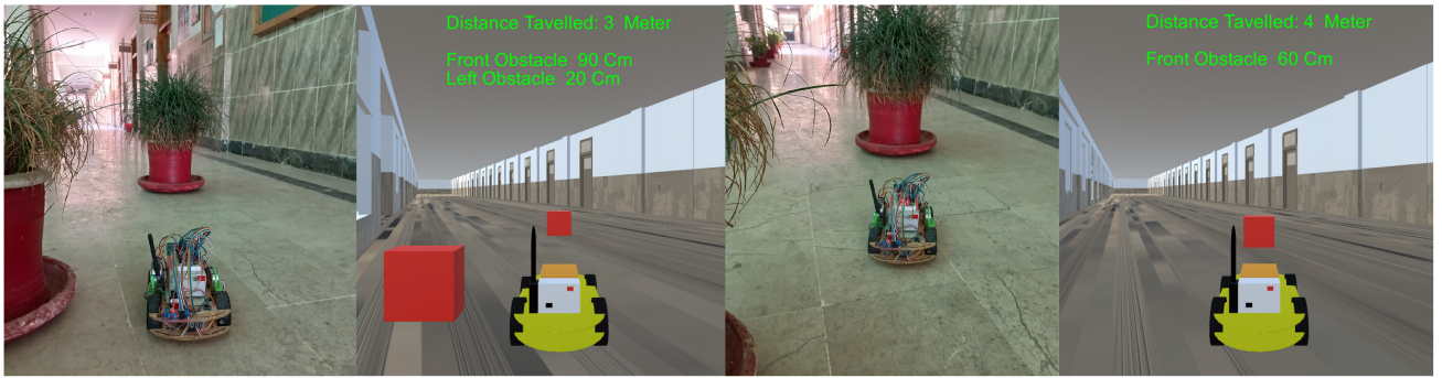
Fig. 8. Real-time detection and visualization of obstacles during navigation.
