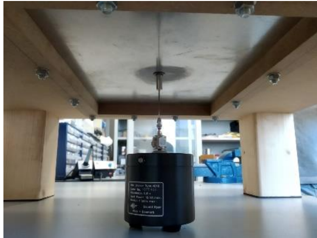
Figure 35. B&K shaker type 4810, connected to the plate via stinger. The PCB load cell is visible at the top of the shaker.
