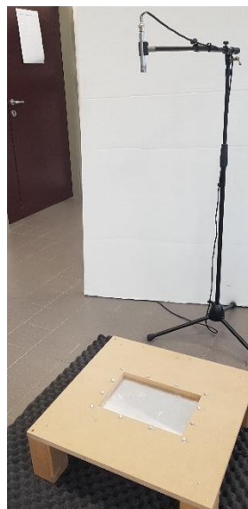
Figure 39. Detail of the B&K microphone mounted over the plate on-axis at 1 meter distance.
