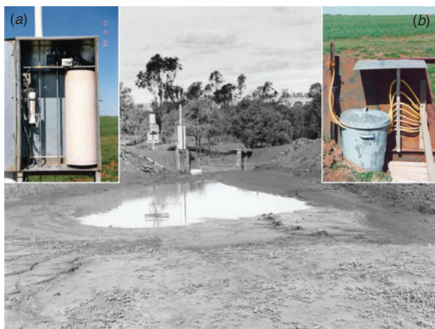
Fig. 4. Photograph of a Cipoletti or trapezoidal weir with bedload collection area in foreground; (a) water level recorder and (b) rising stage water sampler.
