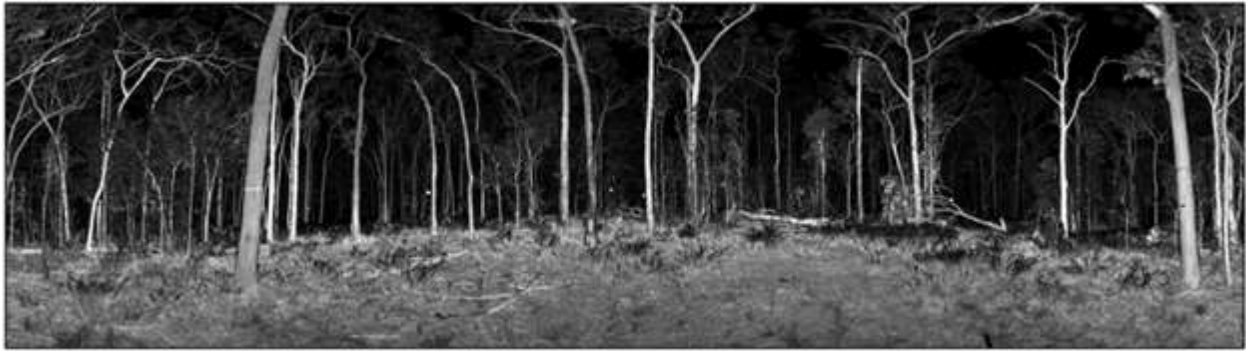
Figure 3-3. Example of terrestrial laser scanning of a woodland community in Queensland. The information collected is a point cloud of spatial (x, y) and return-value (z) coordinates enabling detailed and accurate reconstruction of the three-dimensional structure of the vegetation. A ratio of returned values in the infrared and visible-green wavelengths discriminates denser woody vegetation (trunks and limbs) from leaves and twigs. Image courtesy of the Joint Remote Sensing Research Program.
