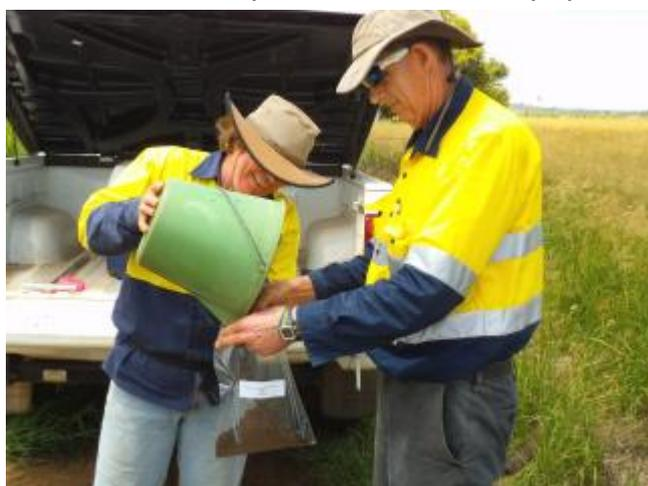
20 soil sample cores (12mm diameter) were taken from each treatment to a depth of 150mm. These cores were bulked and mixed, placed in a plastic bag and samples kept at less than 12°C. The samples were sent to DAF Eco sciences precinct and nematodes extracted from the soil by placing soil on a Baermann tray for 96 h (Whitehead and Hemming 1965). Nematodes were recovered by sieving twice over a 38 µm sieve.
