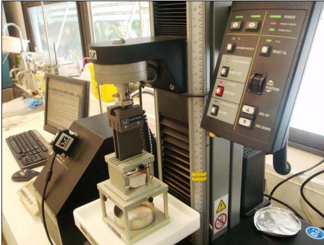
Figure 3. Instron texture analyser with sample loaded into the Kramer-Shear cell
