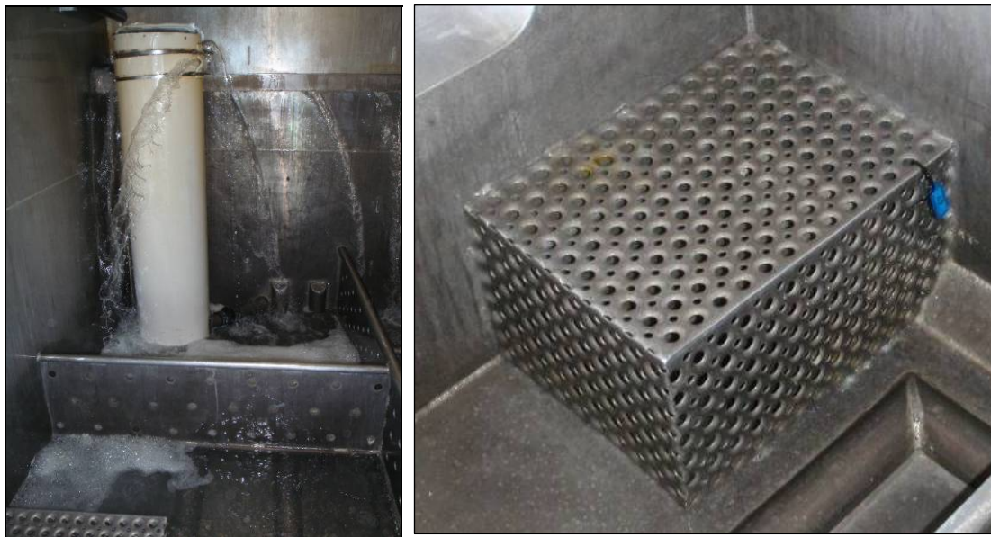
Figure 5. Photographs of brine tank being filled and placement of temperature logger on return cage
